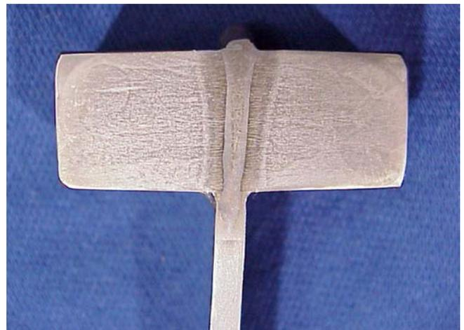
**Fig. 6 EBraze™ Joint in a Compressor Cover**
