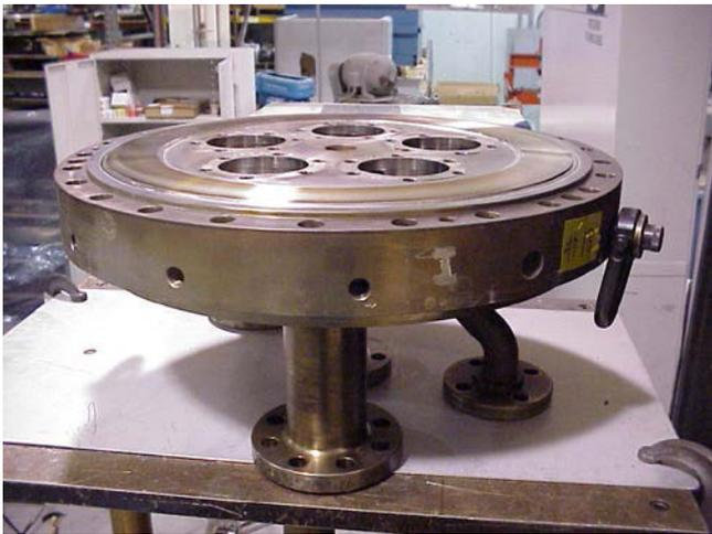
**Fig. 1 Frame 7 Combustor Cover**
