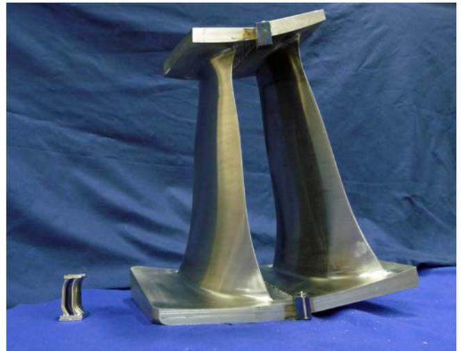
**Fig. 2 W501F Vane Segments After EB Welding**
