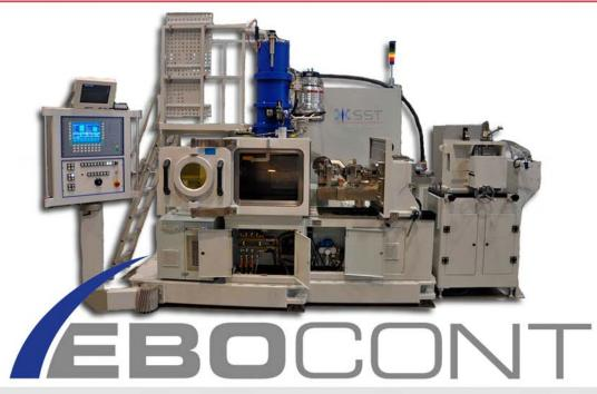
The S7 Electron Beam Welder is used for the high speed continuous EB welding of metal strips. The main uses of these machines are in the electronic industry for contactor materials, resisitors and in the saw-blade industry where high-speed steel is welded to spring steel support strips for various saw blades. The process and parameters are continuously closed loop controlled to produce the highest quality Bi- and Tri-metal welds.
