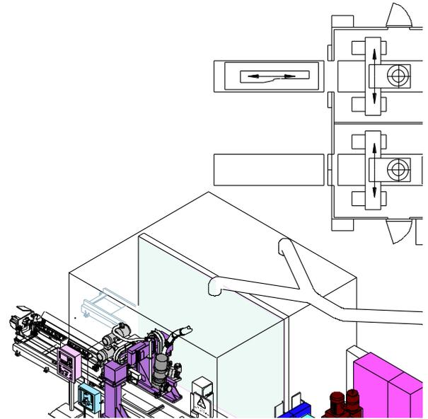
In general the machine layout consists of two separate welding cells each with one linear movement for workpiece and a manipulator for the generator column but with one high voltage supply HVPS together, control cabinet, fume extraction and other auxiliary aggregates.
