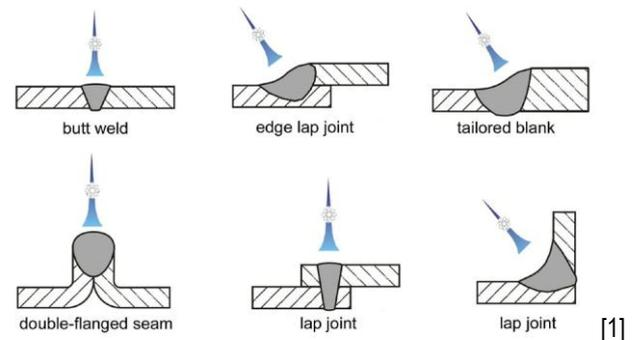
The „Tailored Blank“ joint allows gaps of a few 1/10 mm. In case of a butt weld gaps with < 1/10 mm are tolerated only.
