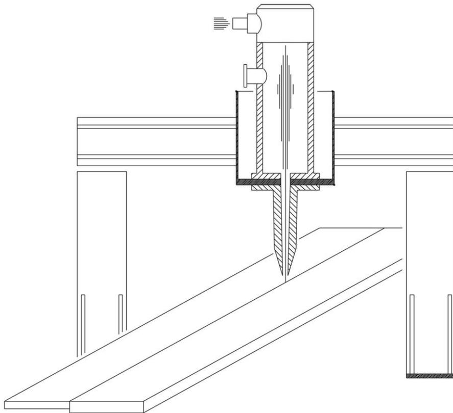
***Electron beam welding
