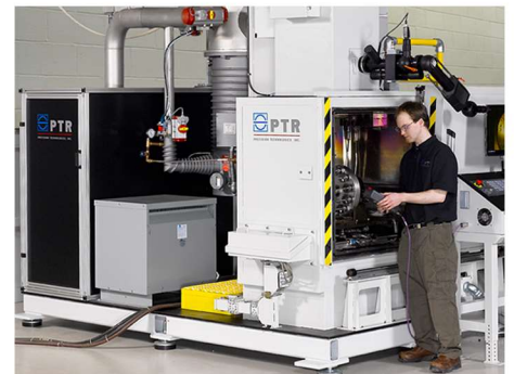
Job Shop EB Welding system with full CNC control & multi-spindle fixture.
